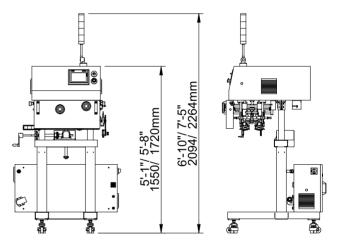
The dimensions shown are for standard machine. The conveyor can be extended: the length may vary based on selected options. This machine can run independently or be integrated into an automated packaging line. All CVC equipment is covered by a one-year parts warranty. Full Warranty details are included in our equipment proposals or can be found on our website.
